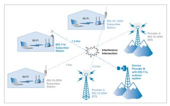
The popularity of Wi-Fi has led to the emergence of many Wi-Fi hotspots and WLANs. These large deployments have some operators concerned about the coexistence of WiMAX and Wi-Fi. A WiMAX license-exempt solution can operate in close proximity to a Wi-Fi network as long as channels are available and proper network design methods have been used. WiMAX enables providers to offer extended wired and Wi-Fi coverage in cities more economically and with wider coverage than with just Wi-Fi alone.
